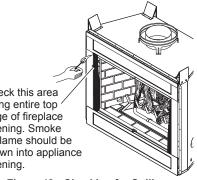
Check this area along entire top edge of fireplace opening. Smoke or flame should be drawn into appliance opening.
